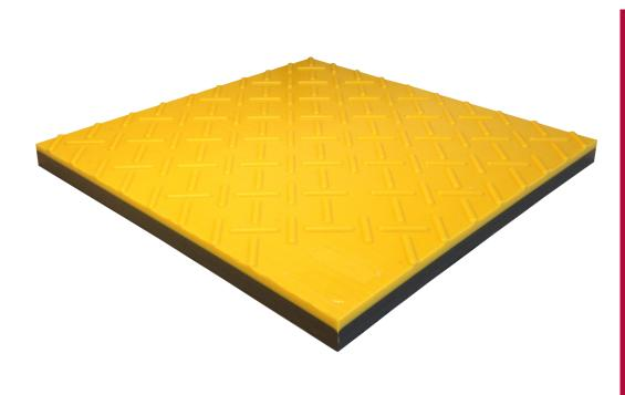
Designed provide to economical and ergonomic solutions for shielding sources below. Each tile combines the attenuation properties of T-Flex® with the durability of a work mat. They also can be cut for in field adjustments. The floor shielding features a non-slip diamond tread surface.
