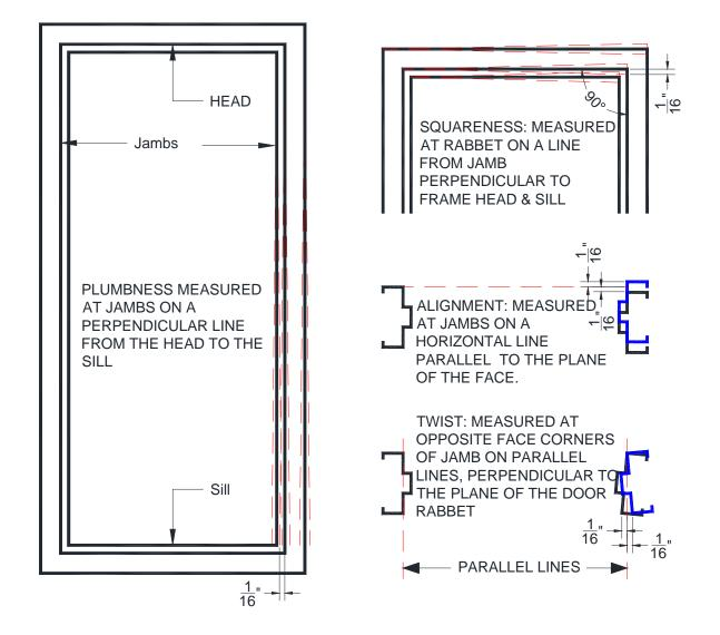
The installation contractor shall have a plumb bob, carpenter level and builder's square. Level the head by positioning the level to the head of the window rabbet. With builder's square, check frame for squareness and twist. Position square against jambs and head and sills at glass rabbet to check for square, adjust as required. Position square against door rabbet and project line perpendicular to the plane of the door rabbet, adjust as required.
