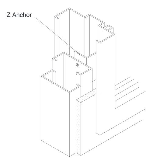
Proper frame anchoring is vitally important to the proper performance of the door opening. A variety of jamb wall anchors are available to suit the various types of wall construction. We are only covering anchors for fixed welded window frames with steel studs in this document.
