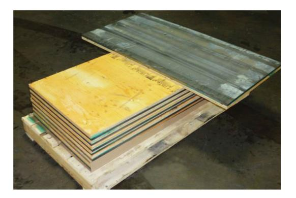
**MarShield** plywood is laminated with sheet lead that is designed to cover necessary surfaces or walls in a room requiring radiation shielding. Lead-lined plywood is ideal for a variety of applications, including new construction or shielding upgrade/renovations for P.E.T and other types of diagnostic imaging rooms, or add additional protection between lead-lined drywall and interlocking lead bricks.
